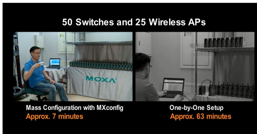
Figure 1: According to Moxa's own lab tests, MXconfig can significantly reduce the initial setup time compared with the traditional hands-on, one-at-a-time approach ( click to watch a demo video ).
